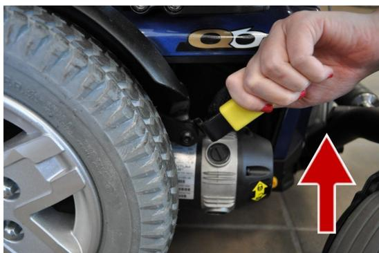
Pulling these handles up **(Figure 4)** will put the motors in "Drive" mode (indicated by a yellow "D" written on the image of a black lock, shown on the sticker that's located on the side of the motor, toward its rear).
