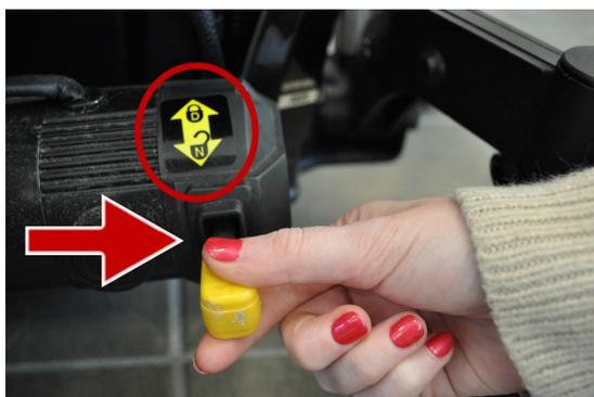
If your motor's switch looks like a yellow nub (**Figure 1**), and it is in the upward position, it will be in "Drive" mode (indicated on the sticker, **circled in red**, that's located above the switch, which shows a yellow "D" written on the image of a black lock).
