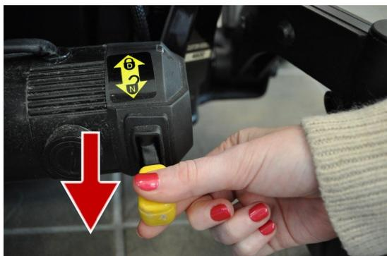
By pressing the switch down (**Figure 2**), the motor will change to "Free Wheel" mode (indicated on the sticker that's located above the switch, which shows a yellow "N" written on the image of an opened, black lock).
