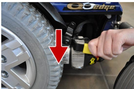
Pushing down on the yellow handles **(Figure 5)** will put the motors in "Free Wheel" mode (indicated by a yellow "N" written on the image of a black lock, shown on the sticker that's located on the side of the motor, toward its rear).
